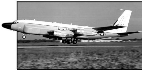
The hog-nosed RC-135 reconnaissance aircraft, Rivet Joint, with its extensive antennae array, provides vital real-time battle management information to mission planners, commanders and warfighters. Rivet Joint aircraft are among the platforms to which PSTS may be extended.
